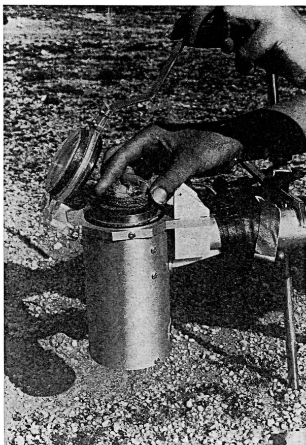
FIGURE 5: Enclosing a lichen sample in the porometer cuvette, the lid of which is opened.
